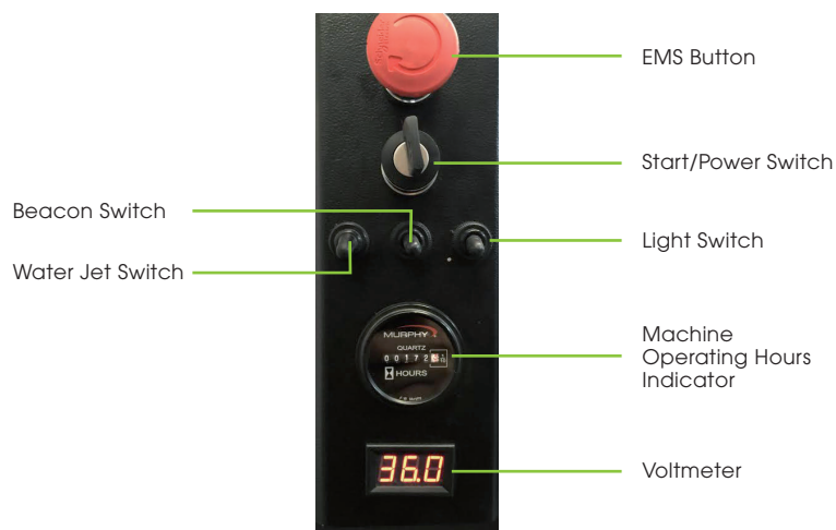
OPERATOR CONTROL PANEL.
